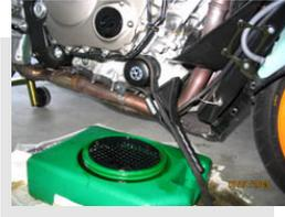
**Don says: Try putting a little oil or grease on the o-ring for spin on filters. For paper filters put some grease on the o-ring to keep them in place when installing. Careful not to pinch the o-ring when doing up the bolts☹**
